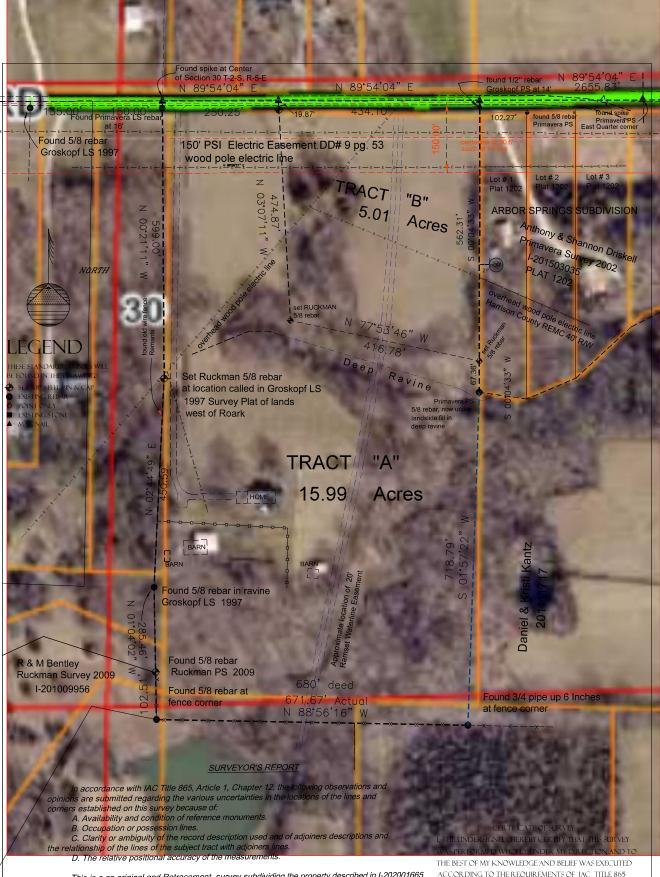
This is a an original and Retracement survey subdividing the property described in I-202001665 of the Floyd County, Indiana records. The basis of bearings shown on this survey plat are per the Indiana State Plane Coordinate System, East Zone using Real-Time Kinematic (RTK) GPS observations INDOT BASE...
